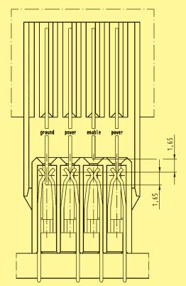
Loaded with four power contacts, each contact can carry up to 20 A @ 70 °C / 80 % derating.
