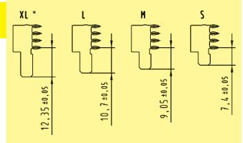
The compact, high temperature moulding can be loaded with up to four high current contacts. Four different contact lengths are available from 7.4 mm to 12.35 mm. This makes sequenced and non sequenced loadings possible (e.g. with GND and ENA). Any other contact assignments, also partially loaded, are available on request.
